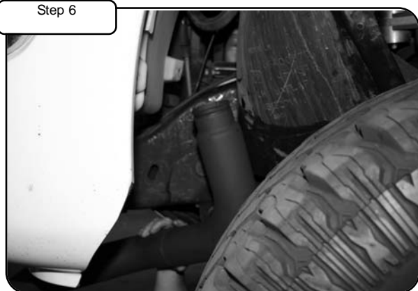
Install the new aFepower intercooler tube through the fenderwell.
