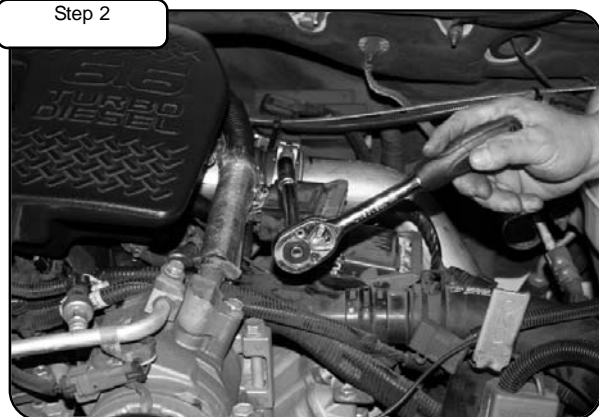
Loosen clamp on intercooler tube using 7/16" deep socket or wrench. Do not damage the coupler hose that attaches to the turbo, as it will be re-used.
