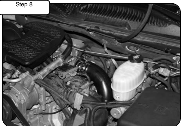
Re-install turbo coupler. Tighten and torque all clamps to 75 in-lbs. Re-install fenderwell. The charge air temperature may reach 400°F at full load. Ensure wiring are routed away from intercooler tube. Your installation is now complete. Thank you for choosing aFepower! Place the included CARB EO sticker on or near the Intercooler Tube on a smooth, clean surface. EO identification label is required to pass the Smog Check Inspection.
